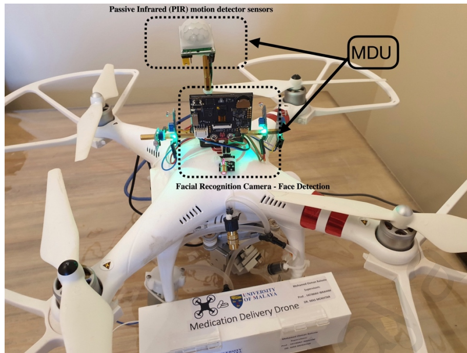
Figure 3.5: Components of Motion Detection Unit (MDU).
