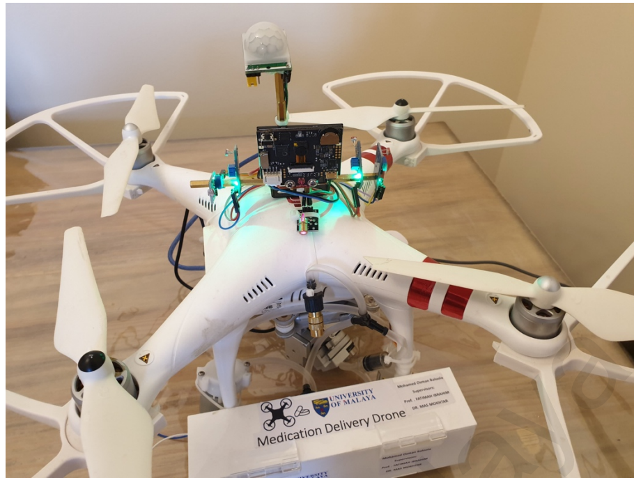
Figure 4.1: UAV with face recognition, Guidance Landing System (GLS) and Delivery Box (DB).
