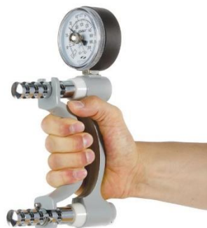
Figure 3.6: Jamar digital hand grip dynamometer for measuring hand grip strength
