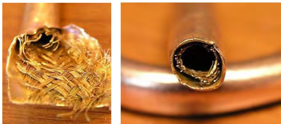
**Figure 2-3: Screen mesh heat pipe.**
