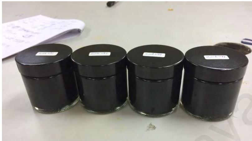
**Figure 3-3: Nanofluid concentrations for sedimentation test**
