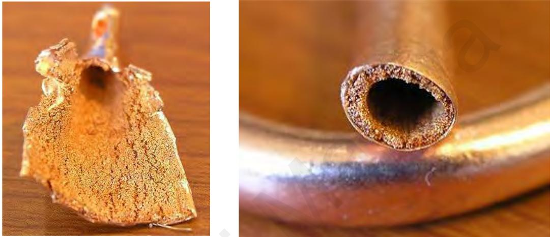
**Figure 2-2: Sintered powder heat pipe (courtesy of Thermal core)**
