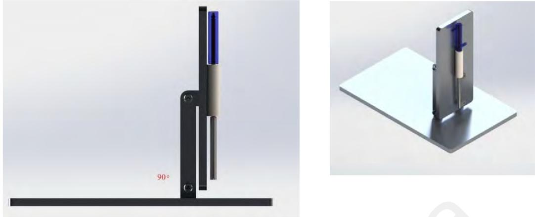
**Figure 3-9: Schematic of the mounting platform with the changeable tilt angle.**
