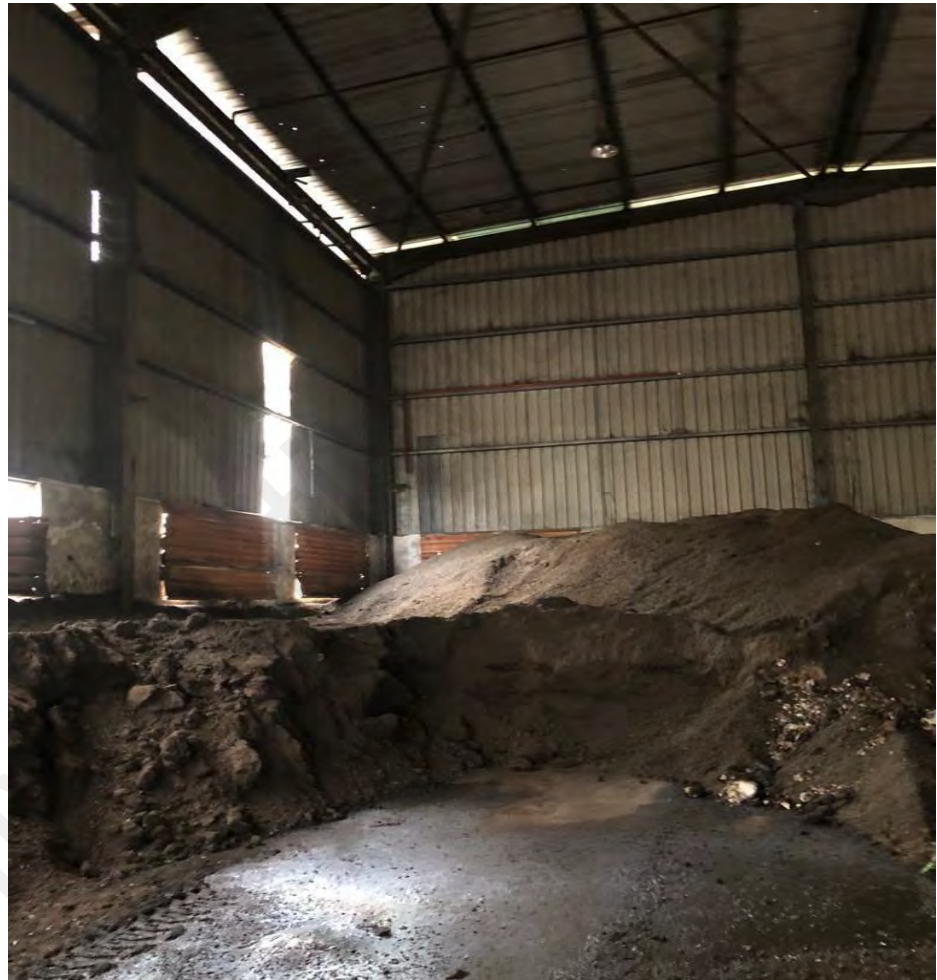
Figure 4.2: Powdered RDF developed in this study
