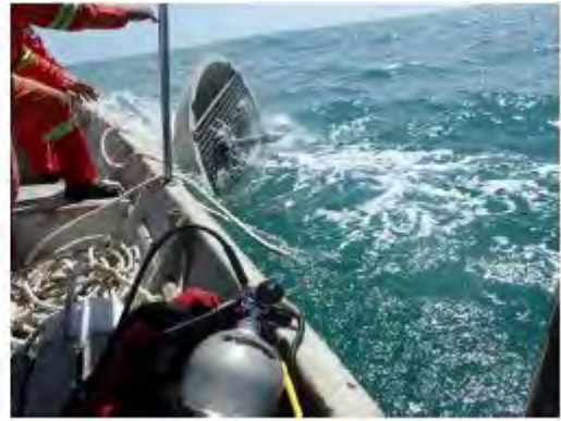
Figure 3.8: The installation and setting up of ADCP at site
