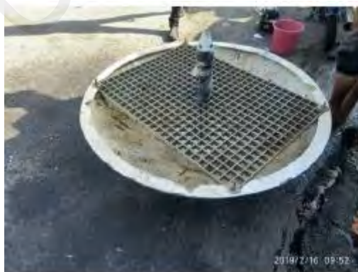
Figure 3.11: Recovered platform and ADCP device
