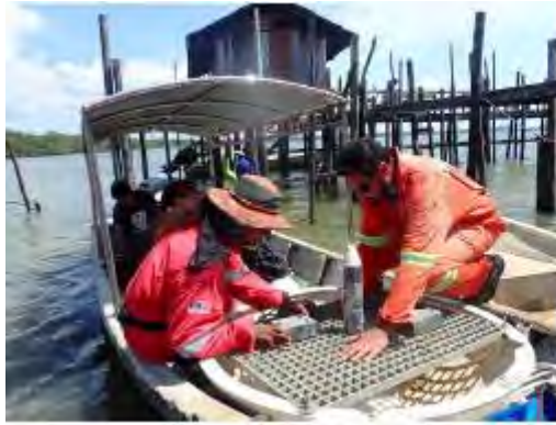
Figure 3.8: The installation and setting up of ADCP at site
