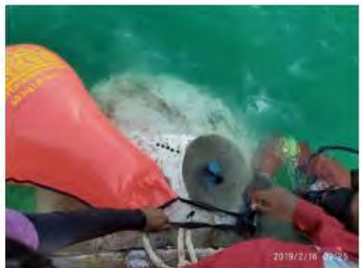
Figure 3.10: Retrieval of ADCP with the aid of Airlift Bag (ALB)
