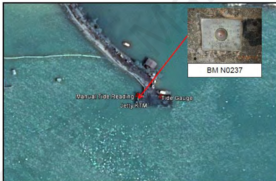
Figure 3.4: Locations of Tidal Gauge and Tide Reading
