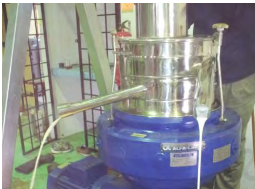
Figure 2.3: The small-scale centrifuge machine used to separate the centrifuged and skim latex (Photo source from www.lgm.gov.my ).
