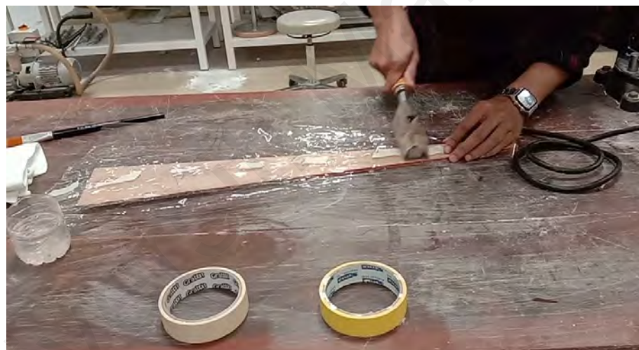
Figure 3.4: PVA Sheet cut according to the size of positive cast
