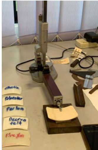
Figure 3.12: Surface testing using Mitutoyo SurfTest SJ-210
