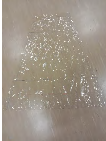
Figure 3.4: PVA Sheet cut according to the size of positive cast
