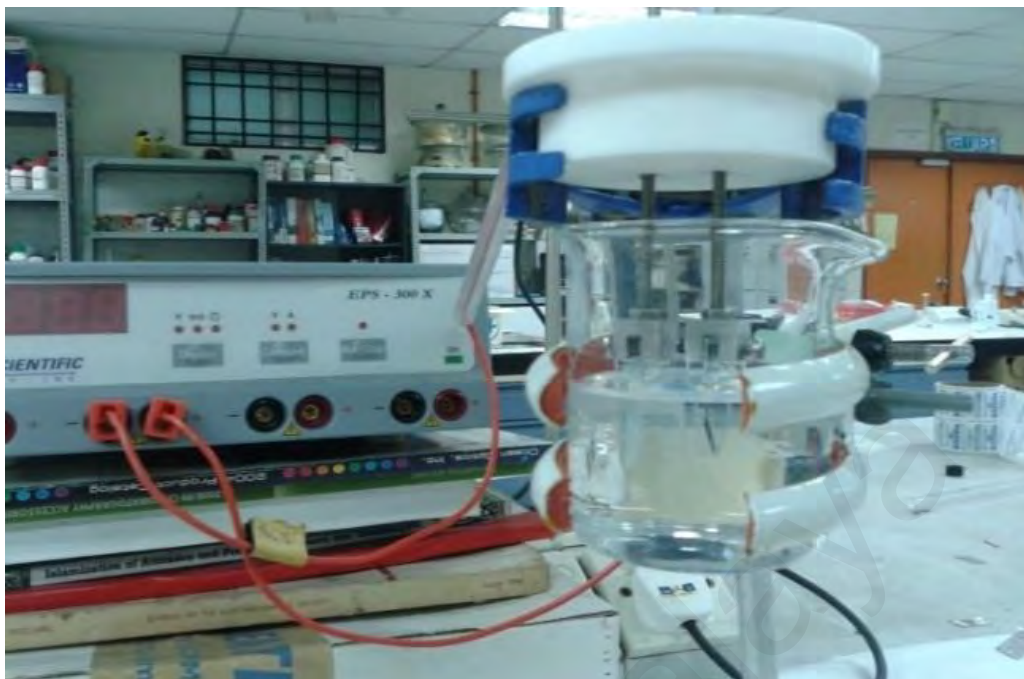
Figure 3.17: Experimental setup for Electrophoresis Deposition (EPD) process showing the control system.
