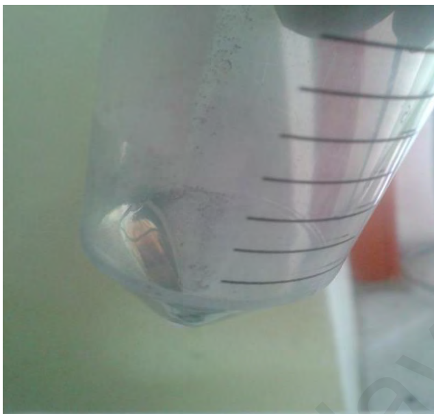
Figure 3.6: Final step of centrifuge process. Shining silver precipitation at the bottom of the 150 mL cylinder.
