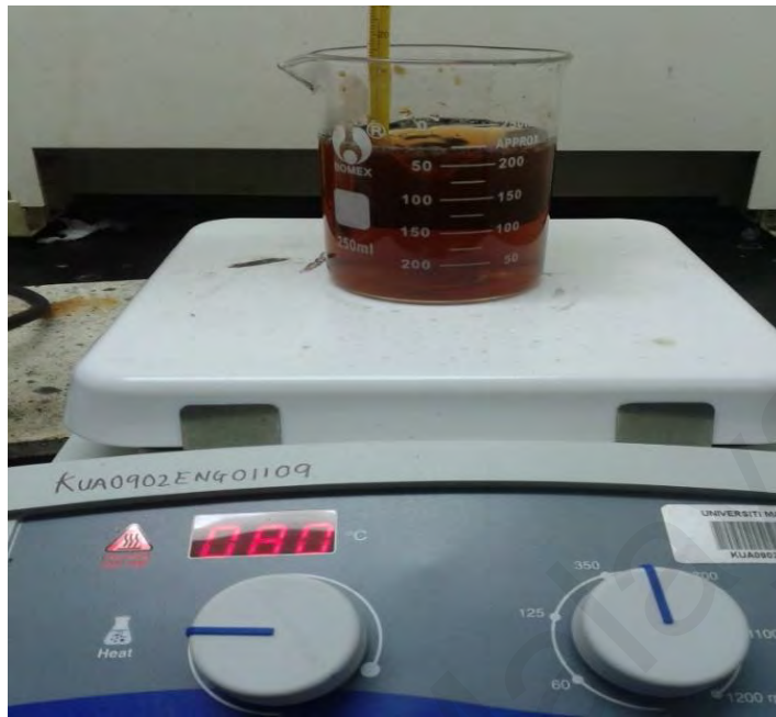
Figure 3.2: Chemical reduction of \text{AgNO}_3 to AgNPs
