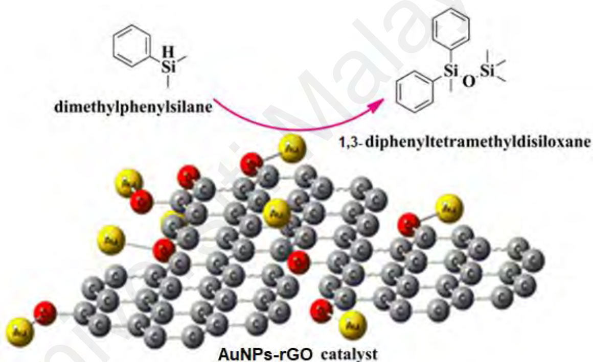
Figure 1.1: Possible arrangement of AuNPs-rGO catalyst.
