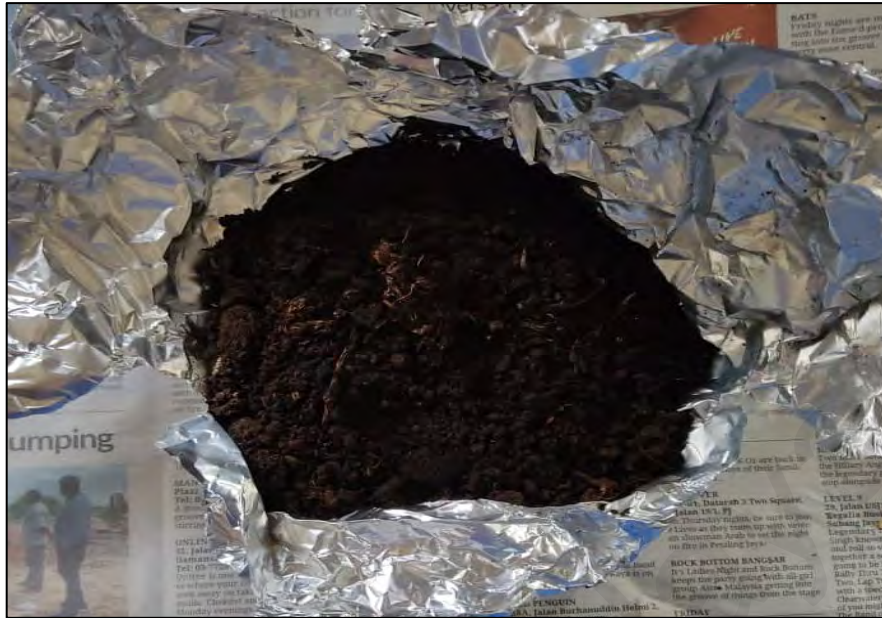
Figure 3.8: Soil samples are dried using oven
