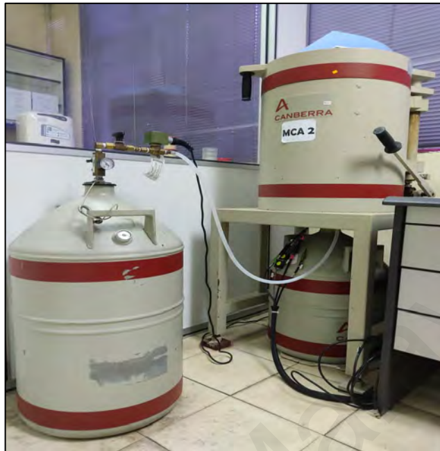
Figure 3.10: HPGe Gamma Detector on the right with the liquid nitrogen tank on the left
