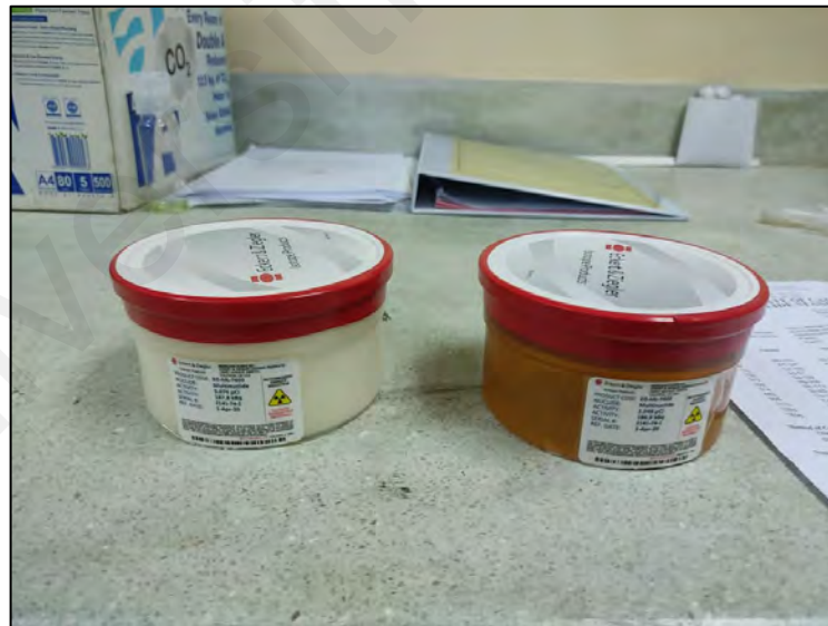
Figure 3.11: Standard radioactive source used to calibrate the detector
