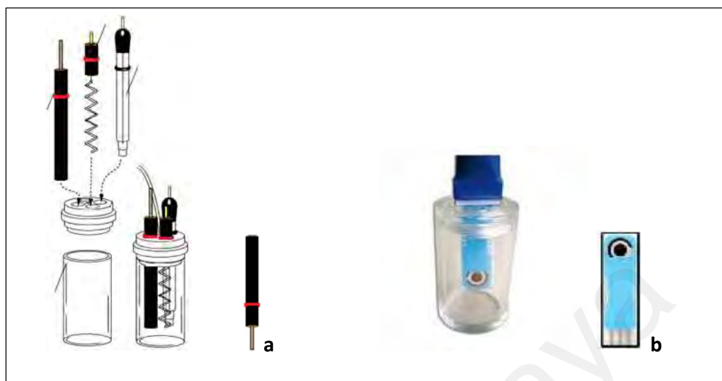
Figure 3.5: Image of the configuration of the electrochemical cell based on the three-electrode system; a) GCE; b) Screen-printed carbon electrode
