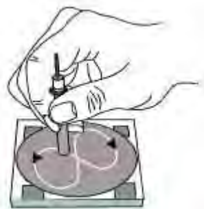
Figure 3.4: Glassy carbon electrode polishing process.
