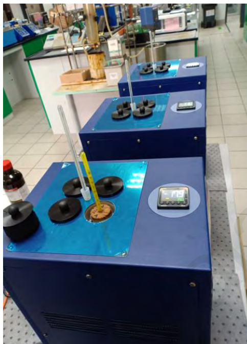
Figure 3.3: Manual cloud point apparatus and cooling bath
