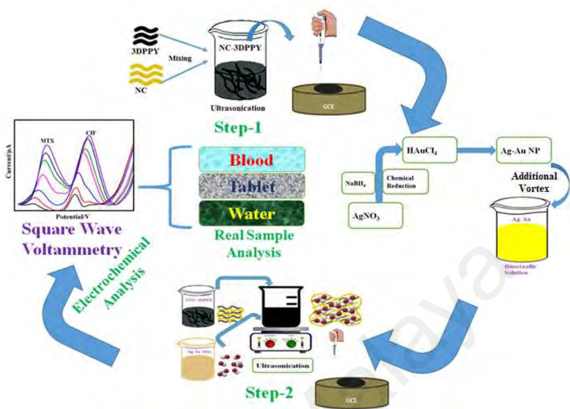
Figure 3.5: Schematic diagram for the preparation of NC-3DPPY@Ag-Au/GCE modified sensor for the electrochemical detection of MTX and ClF.
