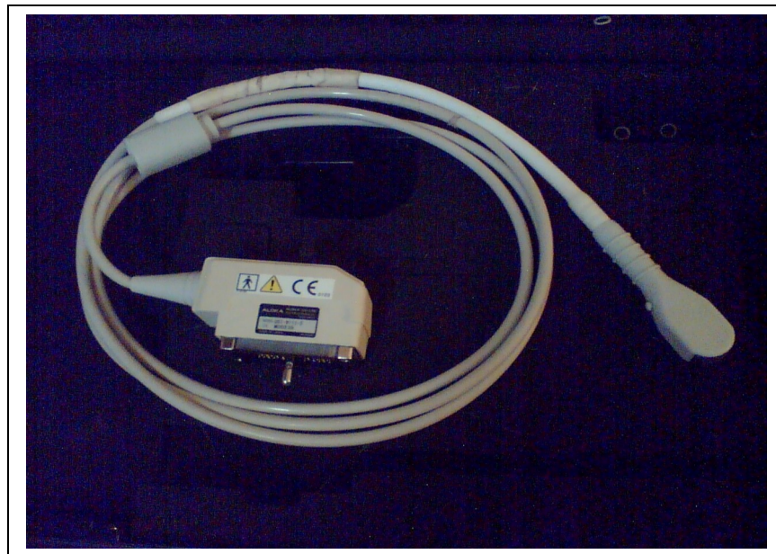
Figure 3.4: Transabdominal probe (5.0 MHz) with 4.0 cm length.
