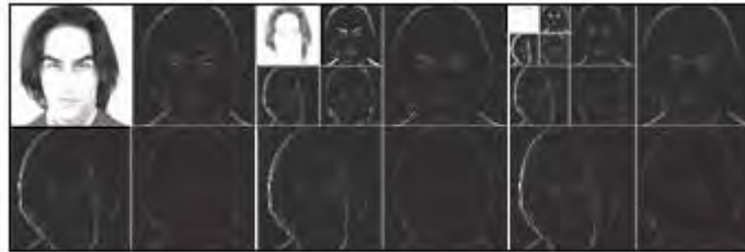
Figure 4.4: Face image with one-level, two-level and three-level wavelet decomposition
