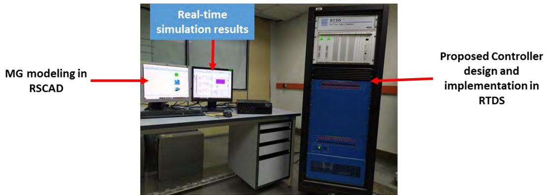
**Figure 4.1: Laboratory setup of the proposed controller for MGs with RTDS**
