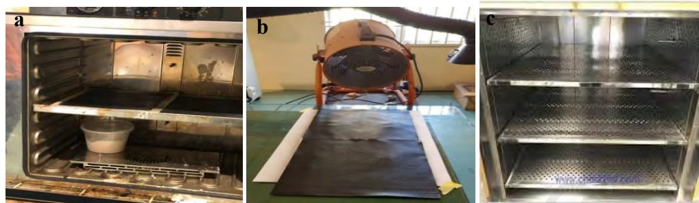
Figure 3.5: (a) Oven and (b) Fan Drying of Carbon Fibre-Epoxy Laminates (c) Hot Air Curing Oven
