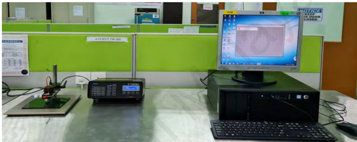
Figure 3.15: Volume Resistivity Testing
