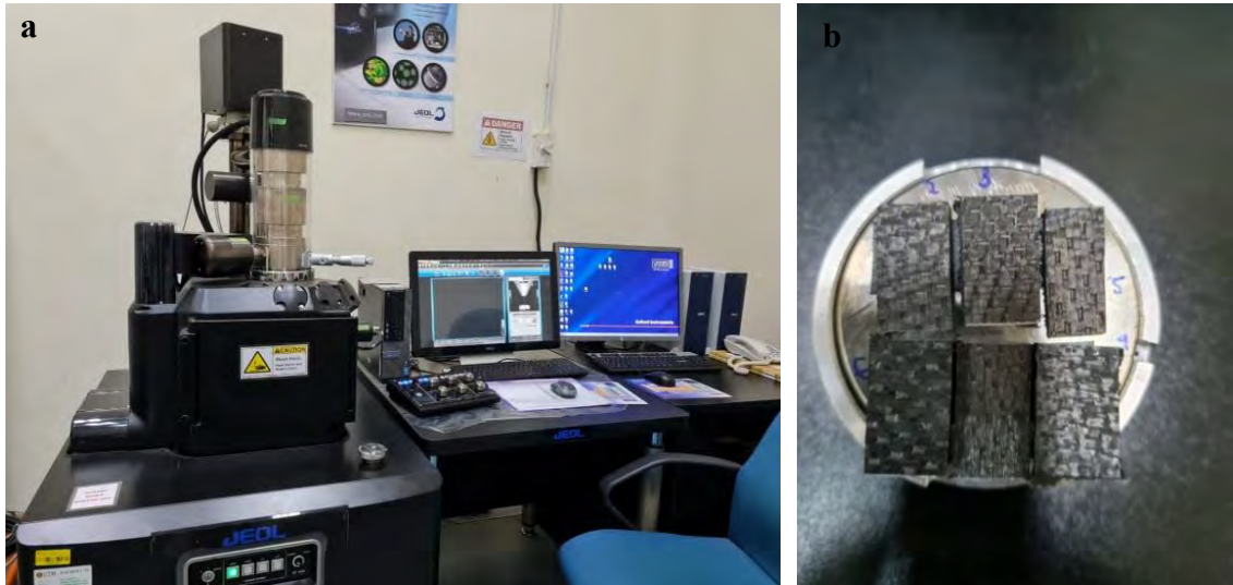
Figure 3.16: (a) Field Emission Scanning Electron Microscope and (b) Analysis of Fractured Surfaces
