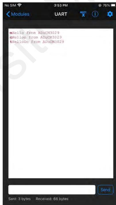
**Figure 4.24: Bluetooth communication between smartphone application and nRF52840**
