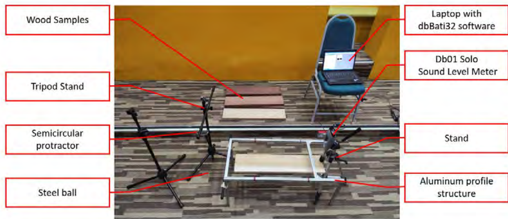
Figure 4.3: Experiment setup for flexural vibration test
