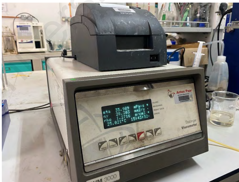
Figure 3.10 SVM 3000 Starbinger viscometer used to measure the viscosity of sugar solution
