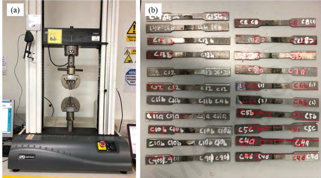
Figure 3.7: (a) INSTRON 3369 universal testing machine and (b) ASTM: E8 standard tensile test specimens
