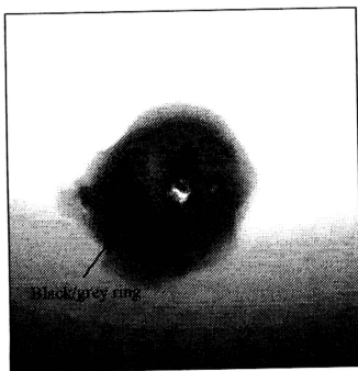
Figure 4.12: The above copper dot has been analyzed by TOF-SIMS to obtain positive secondary ion mass spectra (Scanning area: 500 \times 500 \mu\text{m}^2 ; mass spectra range: 0-500; sampling time: 500 s.)
