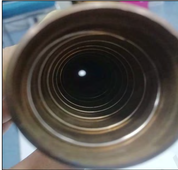
Figure 3.7: Close up wire coil insert in tube
