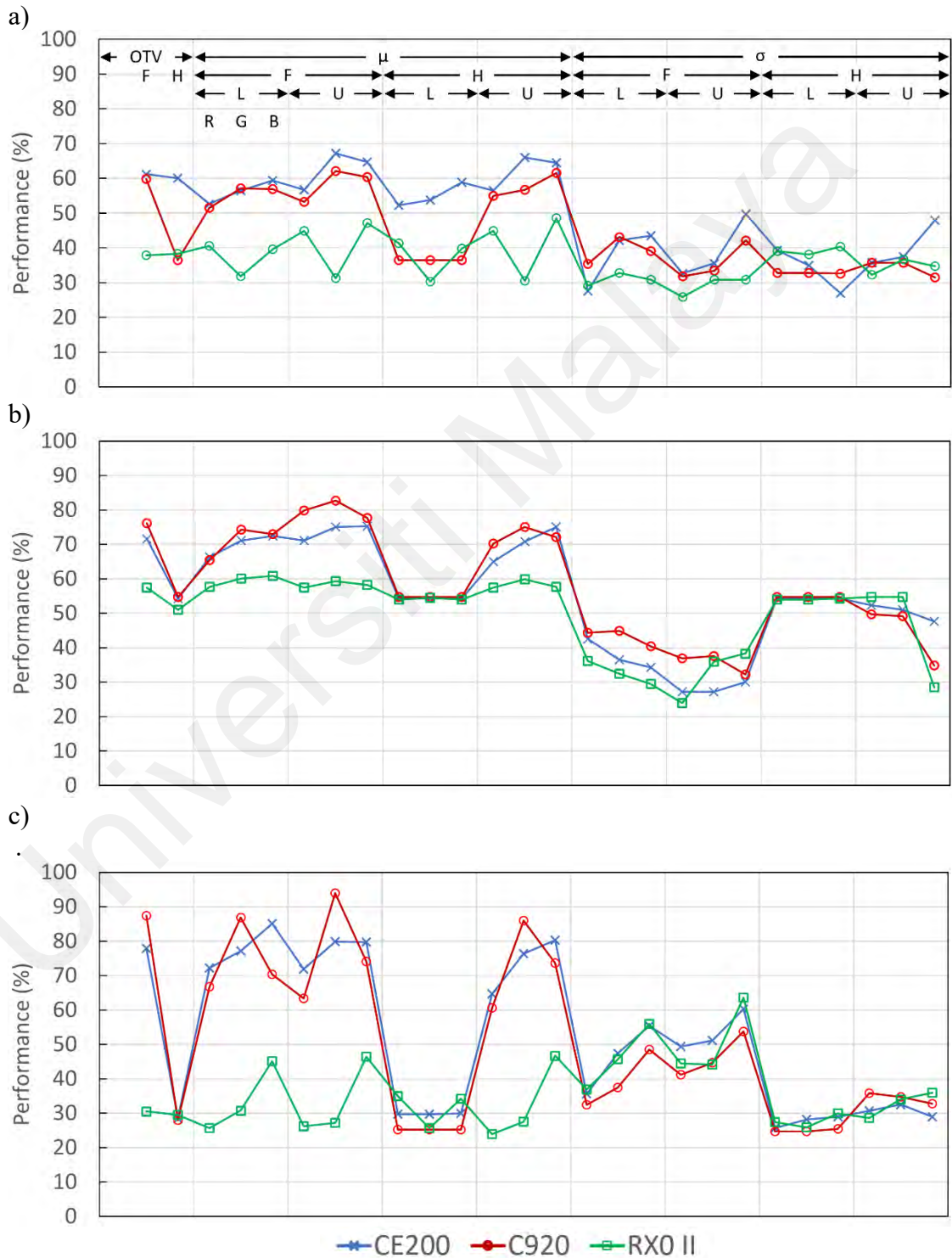
Figure 4.2 The performance of 26 individual features in CE200, C920 and RX0 II for species a) red oak, b) yellow poplar and c) maple, the \mu and \sigma features of each region are arranged orderly in R, G, B triplets.
