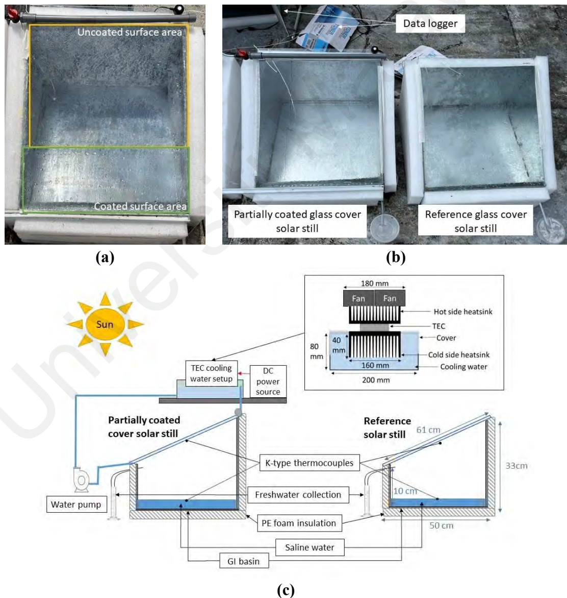
Figure 6.1: Solar still outdoor experimental setup (a) photograph of the partially coated surface with condensate (b) photograph of the setup (c) schematic diagram of the setup.
