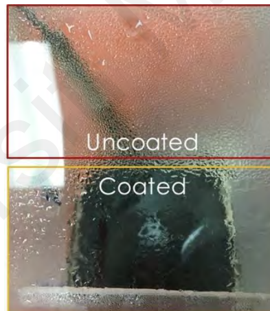
Figure 3.8: Photograph image of coated and uncoated surface for mixed wettability surface of 50% during condensate formation.
