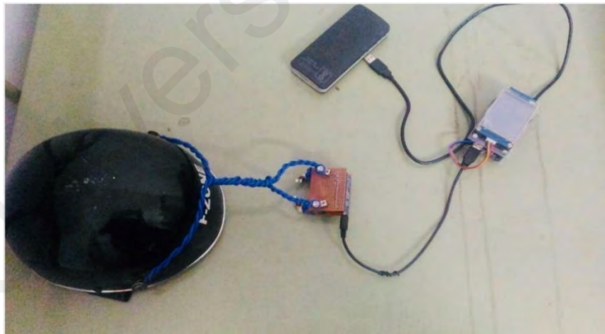
Figure 3.2: Real time architecture of Multi-Channel Speech Enhancement embedded in Helmet
