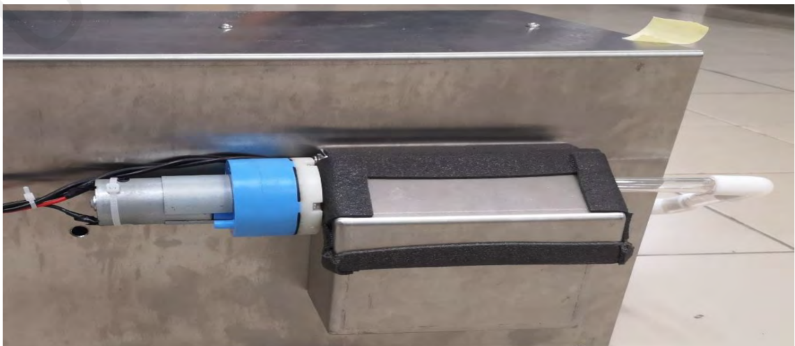
Figure 4.15: Hydrogen peroxide tank covered with foam tape
