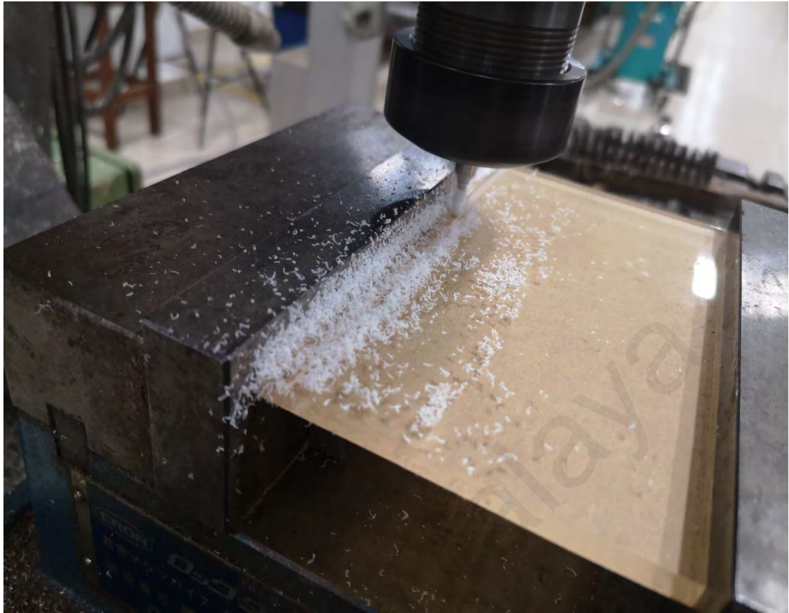
Figure 3.12: Milling a slot in an acryl sheet
