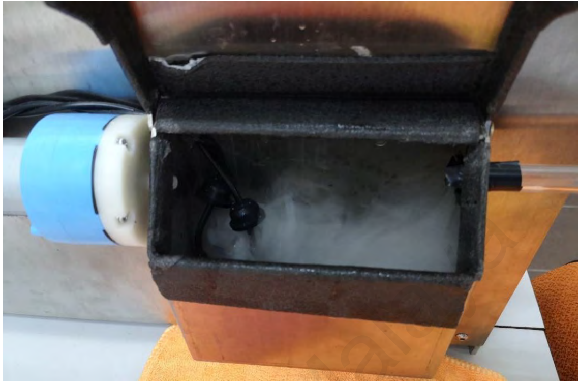
Figure 4.11: Ultrasonic atomizer in operation
