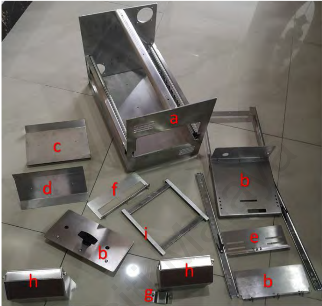
Figure 4.6: Fabricated parts before assembly: a) Frame; b) Drawer assembly, c) Reflector (Above Bulb); d) Reflector (Below Bulb); e) Reflector (Top); f) Reflector (Bottom); g) Lock plate; h) HP tank; i) Jig mounting
