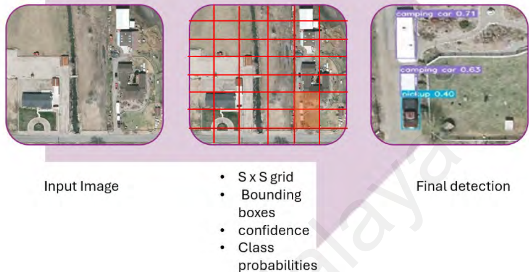
Figure 2.1 General architecture of the YOLO model
