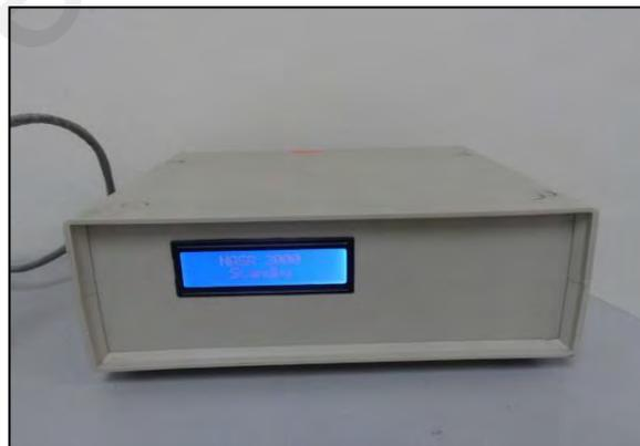
**Figure 3.19:**  $I$ - $V$  tracer (Model: NASA 2.0)
