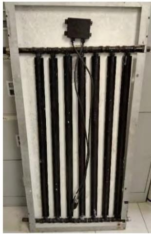
(a) Cooling channel attached to PV backside
