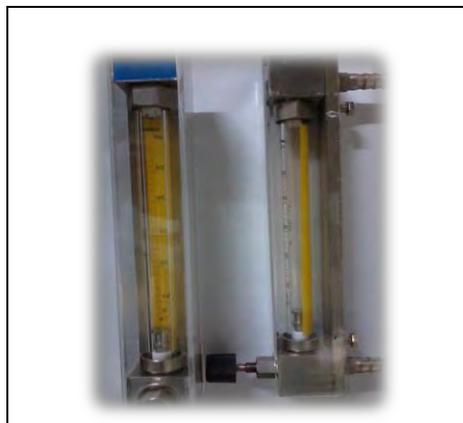
**Figure 3.16:** Flow meter (Model: LZB-10B)
