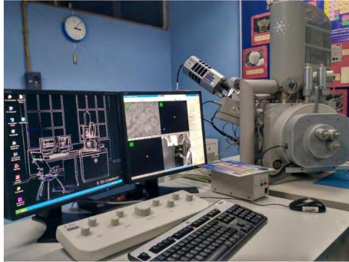
**Figure 3.7:** Field emission scanning electron microscope (FESEM) set up at INFRA lab, Universiti Malaya, Malaysia
