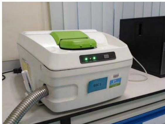
**Figure 3.8:** Differential scanning calorimeter (DSC) at INFRA lab, Universiti Malaya, Malaysia
