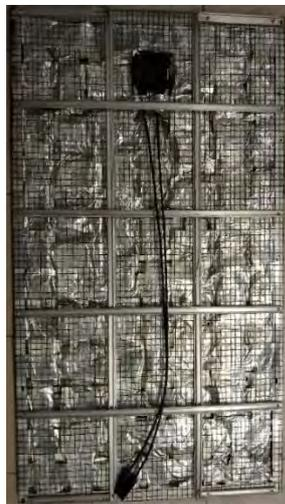
(c) NePCM packets secured by net and aluminum channels
