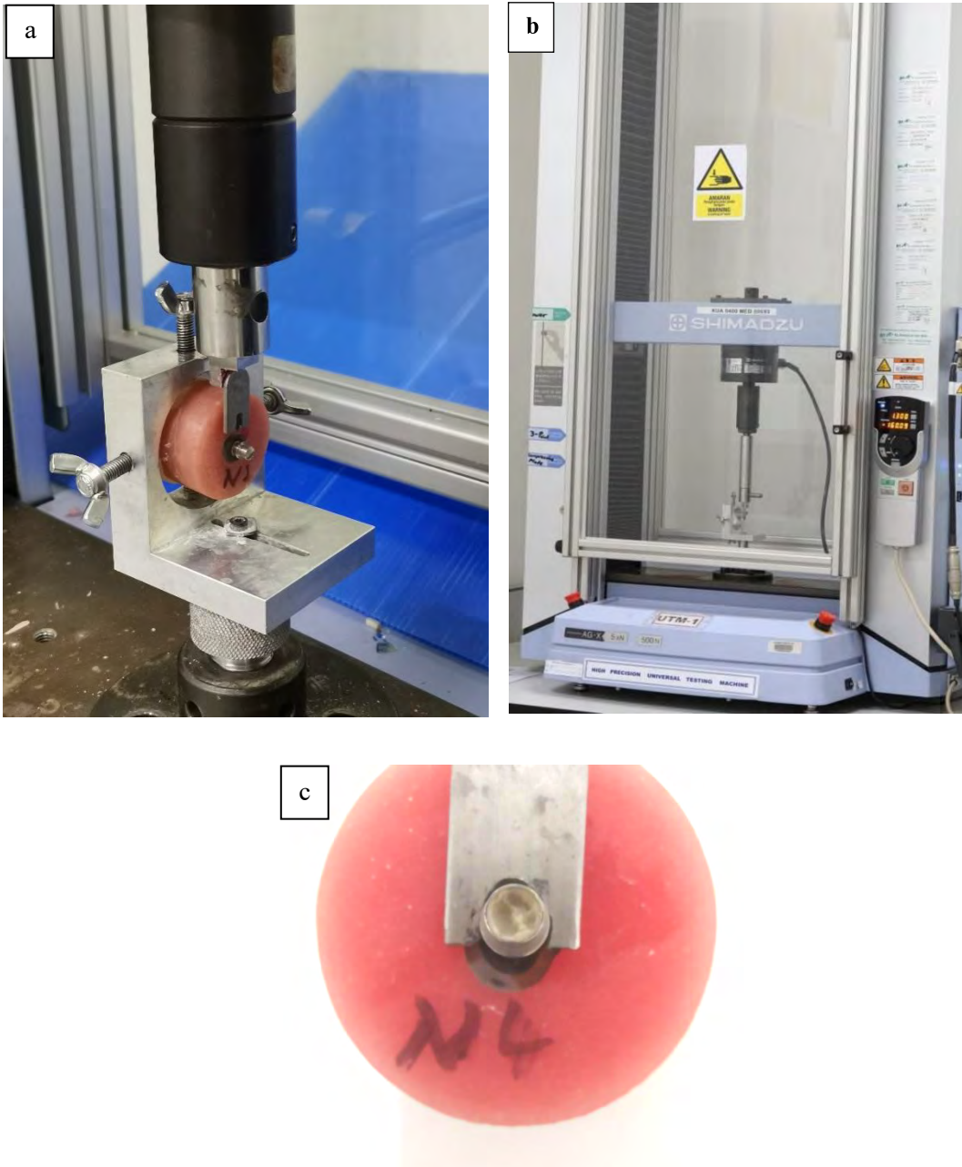
Figure 3.19: a) Universal testing machine (UTM) (Shimadzu, Japan). b) Specimen alignment with the jig in UTM. c) Close-up view of notched-edge jig with metal enclosed mould.
