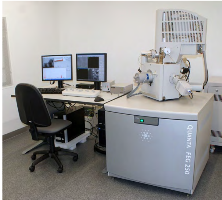
Figure 3.22 Scanning Electron Microscope (SEM) (Quanta-FEG 250, FEI, Germany)
