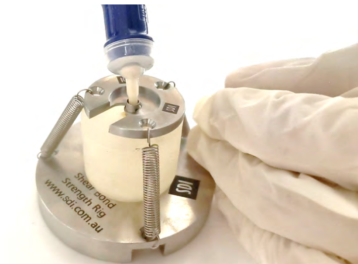
Figure 3.15: Placement of GIC on to the SDI Jig Mould.
