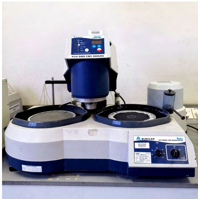
Figure 3.4: Grinding and polishing machine (Isomet, Buehler; Lake Bluff, IL, USA).
