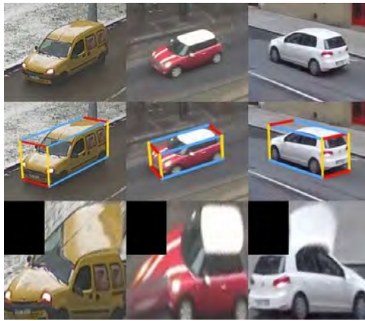
Figure 2.13: Example of Original Vehicles (Top), 3D Bounding Box (Middle) and Unpacked Version (Bottom) (Sochor et al., 2016)
