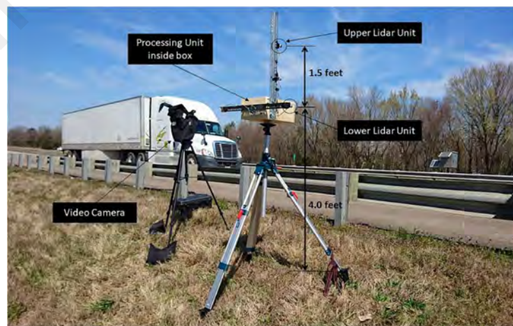
Figure 2.11: Experiment Setup for LiDAR-based VTR (Asborno et al., 2019)
