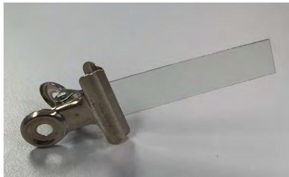
Figure 3.11: Clear surface of indium based coated conductive film substrate
