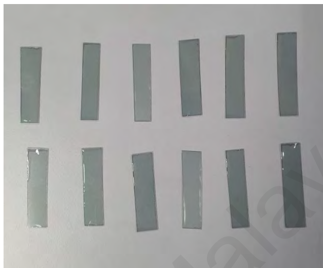
Figure 3.3: 15mm x 25mm size of conductive film substrate
