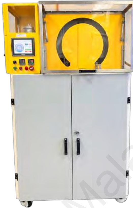
Figure 3.13: Thermocycling machine (Zectron Sdn Bhd, Faculty of Engineering, Universiti Malaya)
