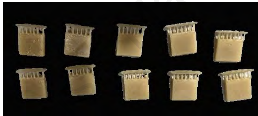
Figure 3.5: 3D printed VSplus samples with the supporting structure
