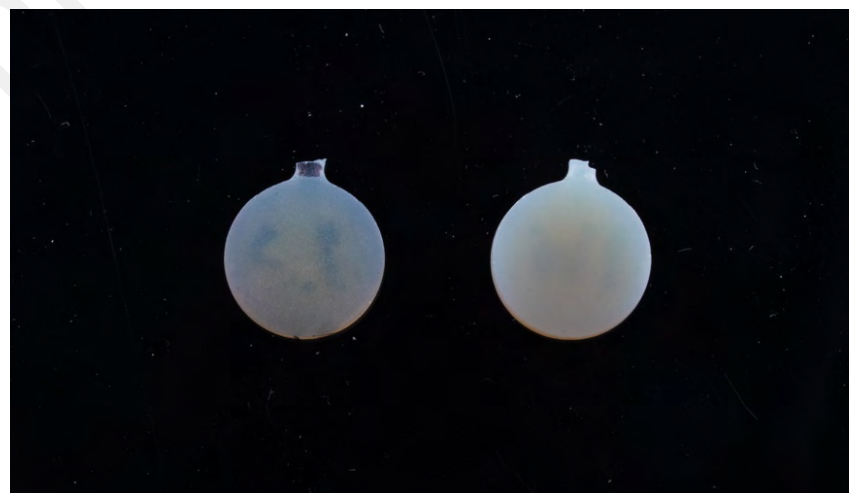
Figure 3.20: Lithium disilicate disc specimens. Left: Pre-crystallized; right: Post-crystallized.
