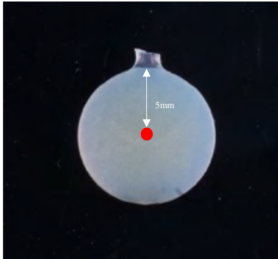
Figure 3.17: SEM images were taken approximately at the centre of each disc.
