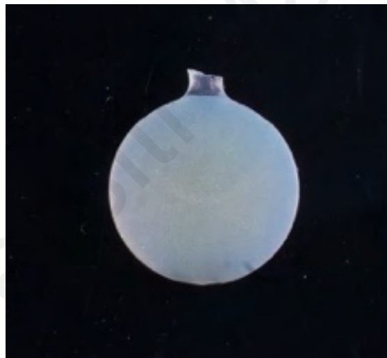
Figure 3.10: Final lithium disilicate disc specimen
