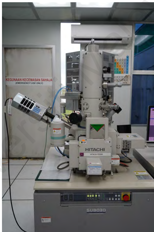
Figure 3.11: Field Emission Scanning Electron Microscopy (SEM) analysis (FE-SEM SU8030, Hitachi)
