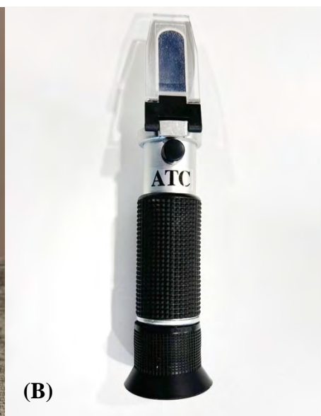
Figure 3.7: (A) Synergy 735 coolant (B) Refractometer
