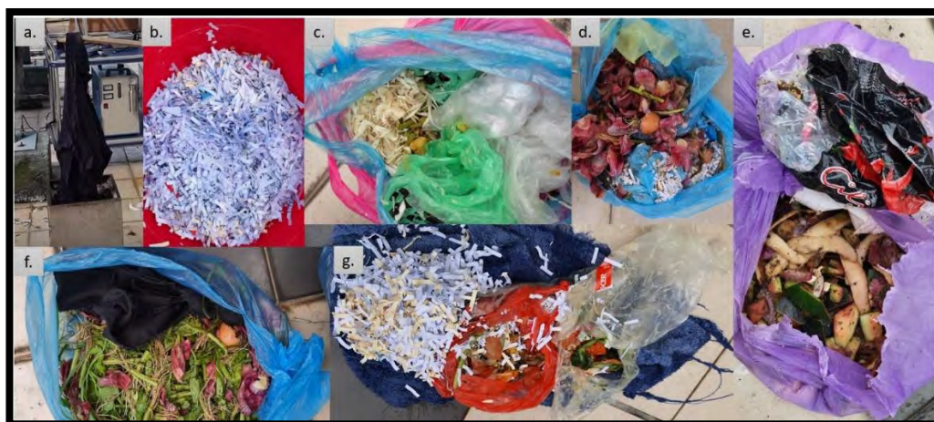
Figure 3.13 Variety of Municipal waste used for incineration test (a) Textile waste; (b) Paper waste; (c) Food waste; (d), (e), (f), (g) Mix waste
