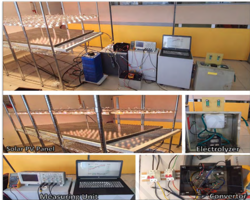
Figure 3.18 Test rig for testing the PV-ELE system, coupled with a DC-DC converter
