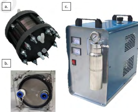
Figure 3.6 Electrolyzer used in study (a) Primary electrolyzer, (b) Secondary electrolyzer, (c) Testing electrolyzer
