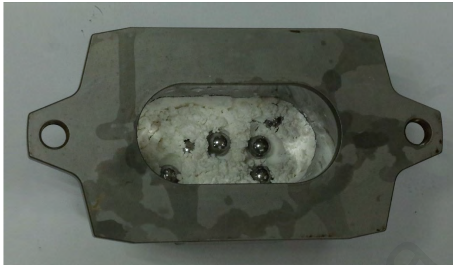
Figure 3.3: MCC and stainless-steel ball in vial before milling process
