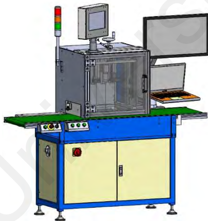
Figure 3.2 a) 3D rendered image and b) actual photograph of the colour sorting machine.
