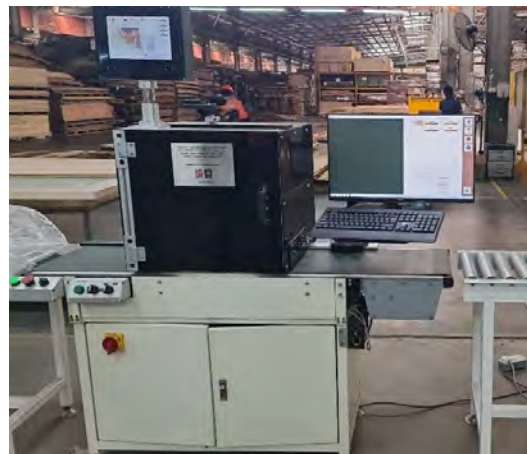
Figure 3.2 a) 3D rendered image and b) actual photograph of the colour sorting machine.
