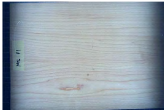
Figure 2.4 Images of the same wavy a) red oak, b) yellow poplar, and c) maple veneers, taken under i) direct lighting (bar light), and ii) a dome light.
