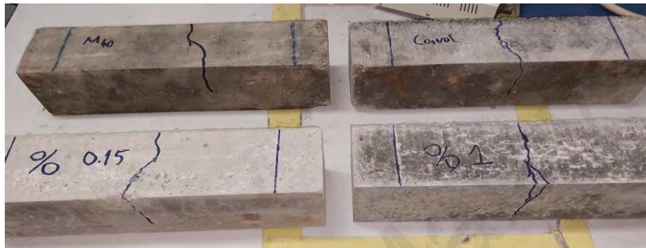
Figure 4.13: Crack propagation of concrete samples after the flexural strength test
