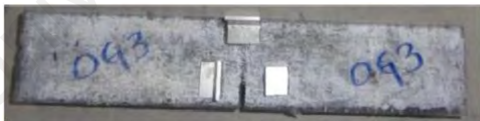
Figure 5.4: Specimens for fracture test
