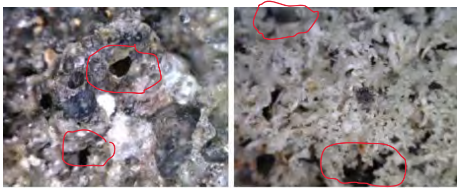
Figure 6.14: Pores in POC
