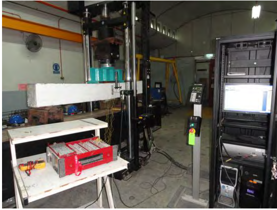
Figure 8.7: Photographs of Beam set-up for flexural test
