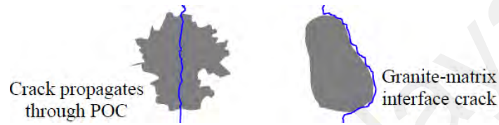
Figure 6.5: Crack propagation schematic diagram for P-GC and G-GC
