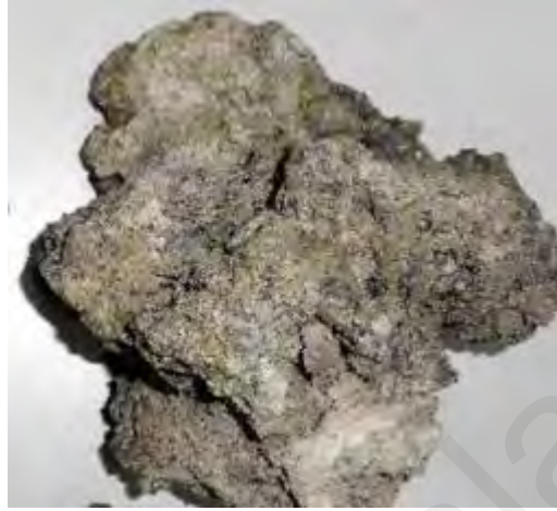
Figure 3.5: Palm oil clinker aggregate (POC)
