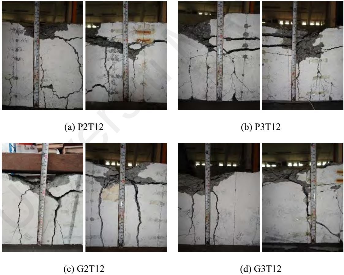
Figure 8.18: Wedge development at ultimate failure
