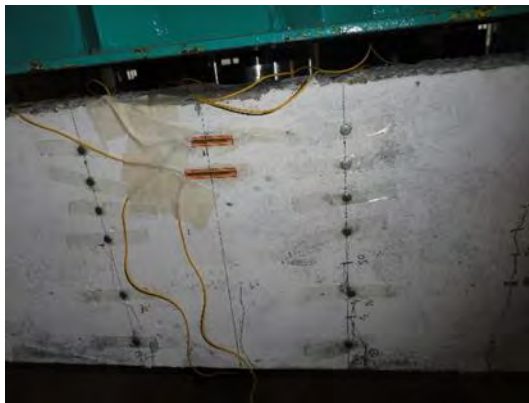
Figure 8.7: Photographs of Beam set-up for flexural test
