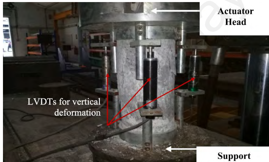
Figure 6.1: Test set-up for compression toughness experiment
