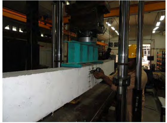
Figure 8.7: Photographs of Beam set-up for flexural test
