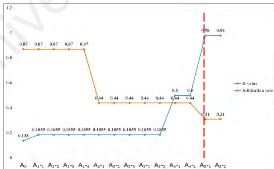
Figure 4.17: The relationships between the infiltration rate and the window settings' combined R-value
