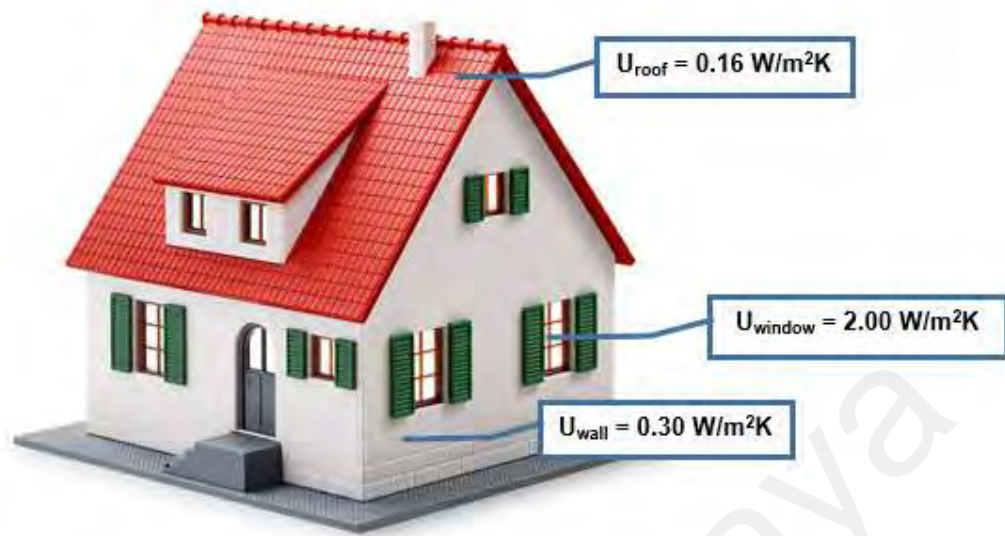
Figure 2.10: Typical u-values of building elements
