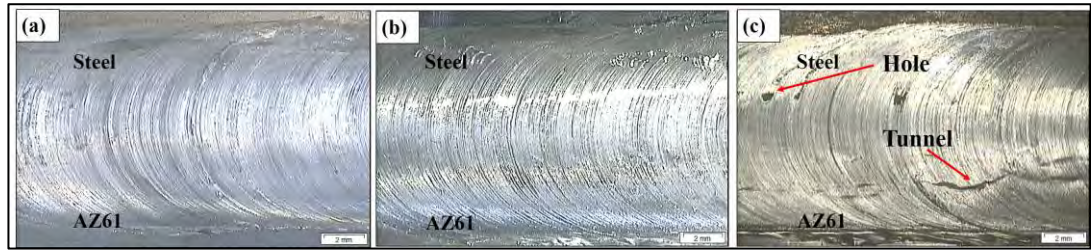
Figure 4.13: The surface appearance of dissimilar friction stir alloy process between AZ61 and mild steel at different welding with 3% CNT additive, at (a) 15 mm/min, (b) 30 mm/min (c) 50 mm/min
