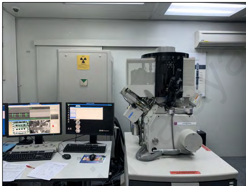
Figure 3.18: Dual-focused ion beam machine for lamella preparation
