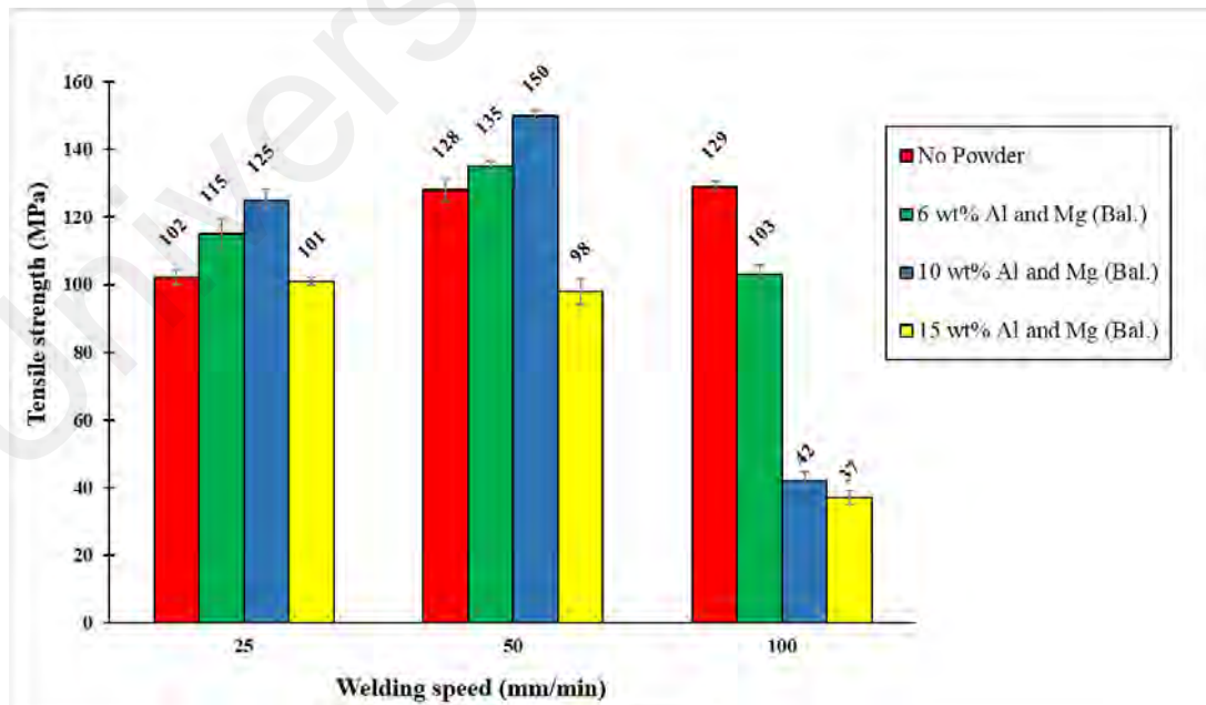
Figure 4.10: Joint strength for different welding speeds and Al powder percentage
