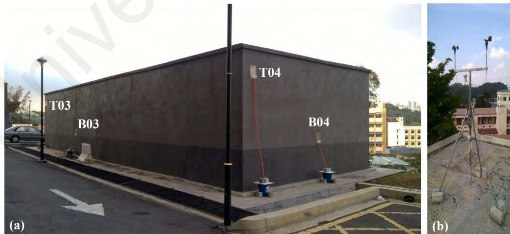
Figure 3.6. The pilot building and position of the WDR gauges on the façades (a) South view (b) Meteorological mast on the rooftop of the building at the parking area.
