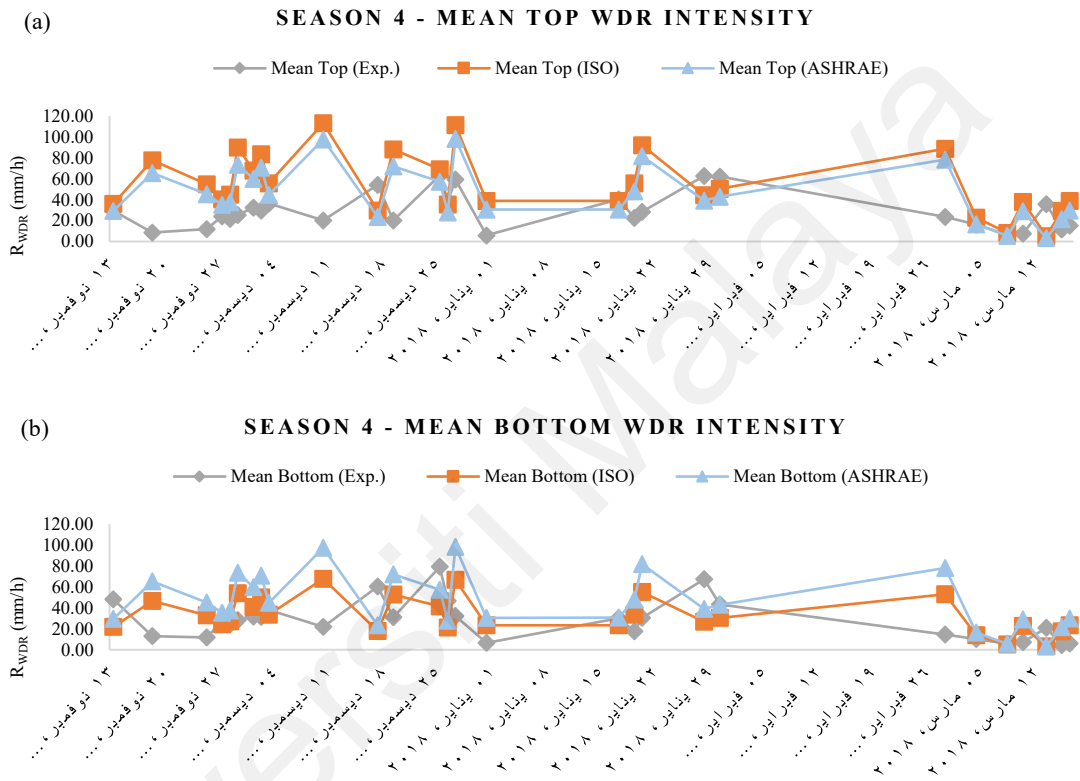
Figure 4.35. Comparison of the Mean R_{wdr} (mm/h) between Experimental measurement and Predicted values using the Proposed WDR coefficients for two positions (Top (a) and Bottom (b)) on the windward façade (NE-NW) – Season Four
