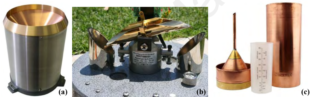
Figure 3.4. Meteorological instruments using by Malaysian Meteorological Department for horizontal rainfall ( S_h ) measurements, (a) tipping bucket, (b) automatic horizontal rain gauges, (c) conventional horizontal rain gauges (MMD, 2024)
