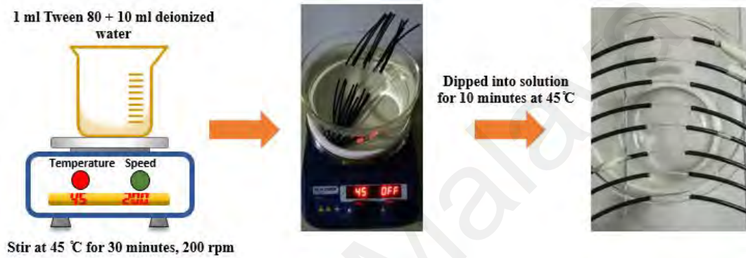
Figure 3.8: POF surface treatment process
