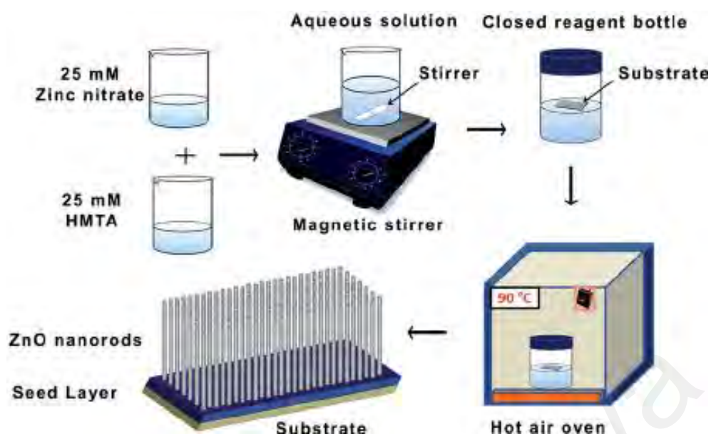
Figure 2.10: Schematic diagram of the procedure for the synthesis of ZnO nanorods using hydrothermally method (Gaddam et al., 2015).
