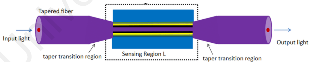
Figure 2.6: A schematic diagram of a tapered optical fiber (D. Wang et al., 2021).
