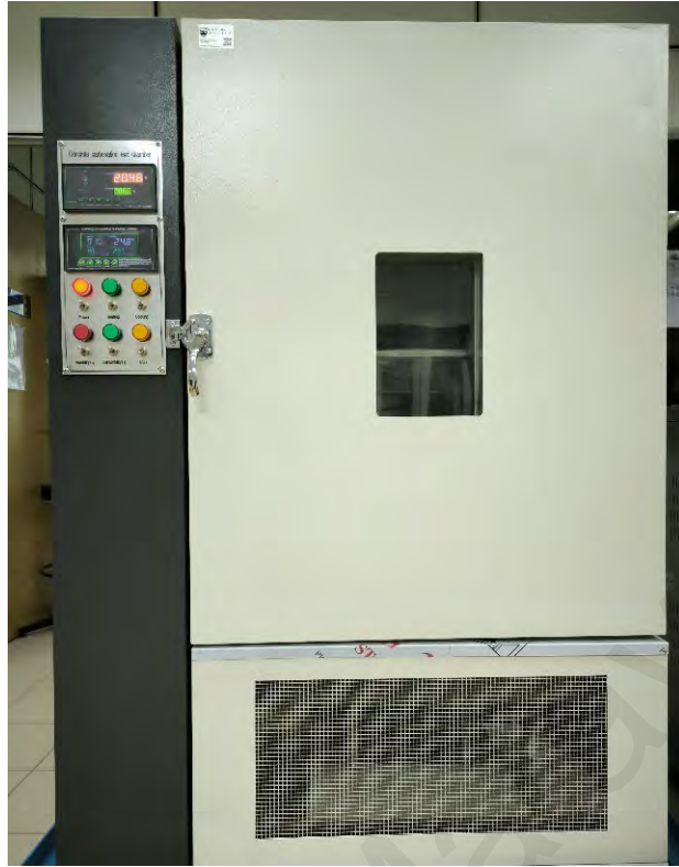
Figure 3.5: Operating carbonation chamber at the set parameters
