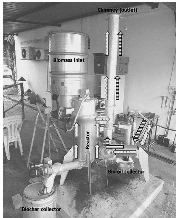
Figure 3.3: The biochar experimenters kit at MPOB, Kajang (Haryati et al., 2018)
