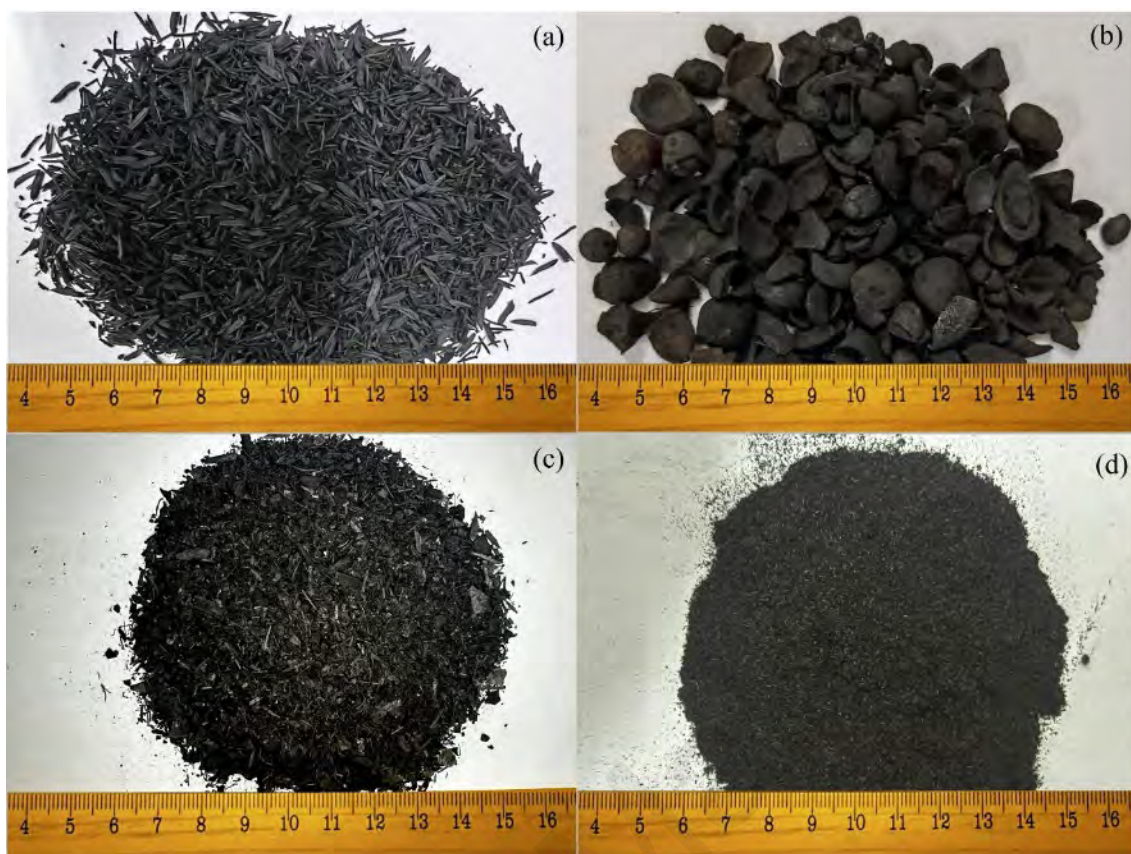
Figure 3.4: Locally obtained biochar (a) RHB (b) PKS (c) CHB (d) BB
