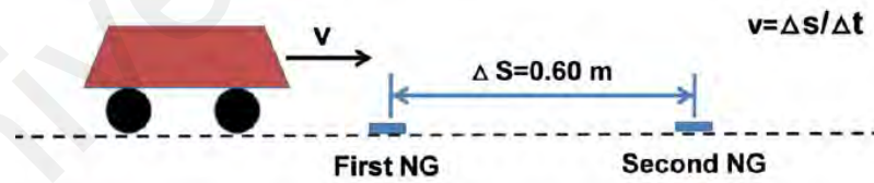
Figure 2.3 Illustration of the working mechanism of a speed sensor (Lin et al., 2013)
