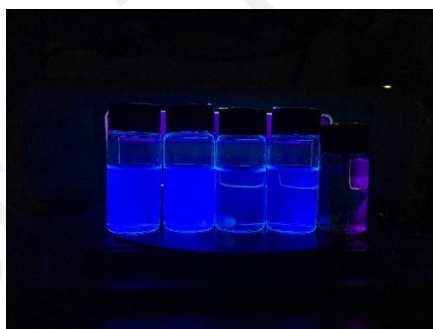
Figure 3.6: Solutions of nanocomposite viewed under UV lamp 365 nm with different weightage percentage. From right, 0, 0.15, 0.25, 0.35 and 0.50 wt% of P(VDF-TrFE) / ZnO QDs.
