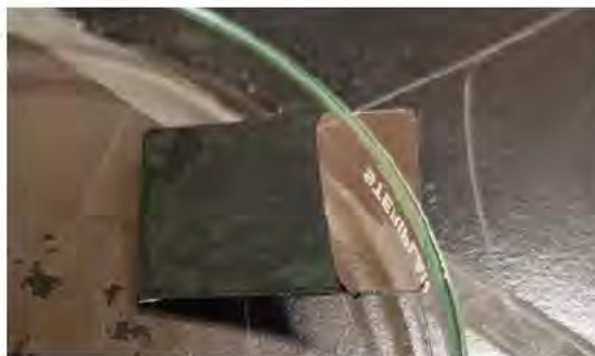
Figure 3.2: Polymeric film deposit on the conductive side of ITO glass piece after electrochemical synthesis.
