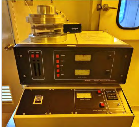
Figure 3.7: Oxygen plasma parallel plate etcher (Polaron PT7170).
