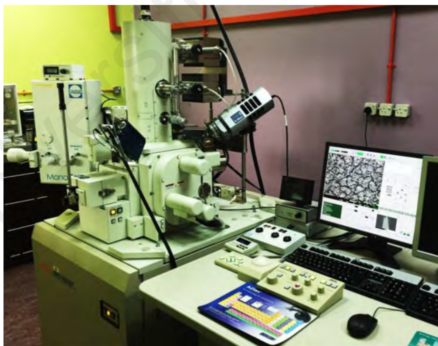
Figure 3.18: Field Emission Scanning Electron Microscope (FESEM) JEOL JSM-7600F.
