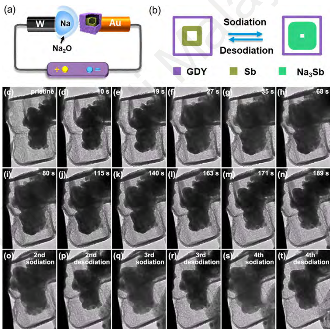
Figure 2.18: (a) Schematic illustration of the in-situ TEM device. (b) Schematic of morphological evolution of hollow yolk-shell Sb@Void@GDY NBs during sodiation/desodiation. (c-t) In-situ TEM images from a time-lapse video of the first four sodiation/desodiation cycles. (Yan Liu et al., 2023)
