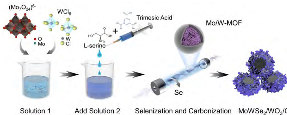
Figure 4.35: (a) Schematic illustration of the synthetic route for MoWSe 2 /WO 3 /C.
