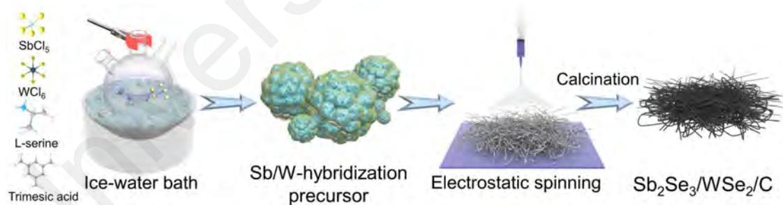
Figure 6.26: Schematic illustration of the synthetic process of the \text{Sb}_2\text{Se}_3/\text{WSe}_2/\text{C} .
