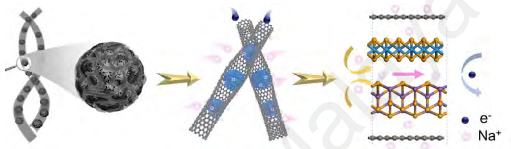
Figure 6.48: The schematic illustration of electron and \text{Na}^+ transfer behaviors in \text{SbWSe} heterostructures with dual-carbon composites.
