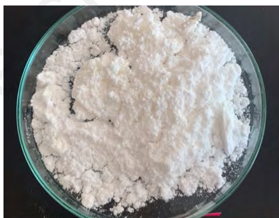
Figure 3.4: P(VA-AA) via alcoholysis.
